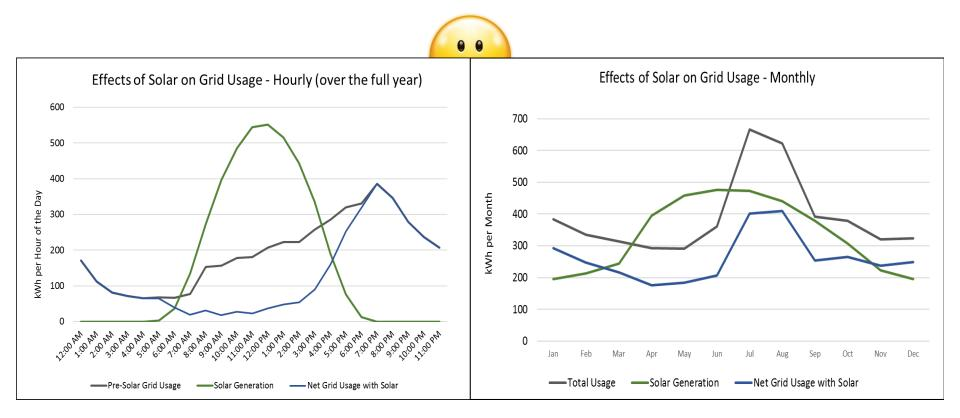
Totals Pre-Solar Grid Usage: 4684 kWh/yr Solar Generation: 4000 kWh/yr (~85% of grid usage) Net Grid Usage with Solar: 3142 kWh/yr (~67% of grid usage) Percent of solar energy used by home ("self-consumption") ≈ 39%
